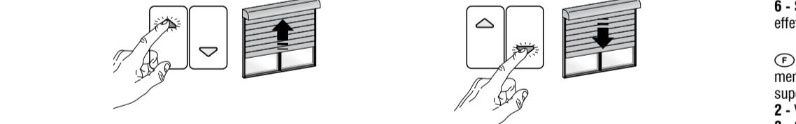
RESET O MODIFICA DEI PUNTI DI ARRESTO IMPOSTATI - RESET OR CHANGE LIMIT SWITCH SETTINGS
